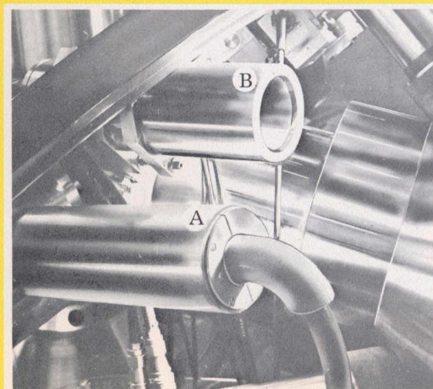
Two x-ray tube mountings, lower (mount "A"), goes through the piston and up to the sample.
